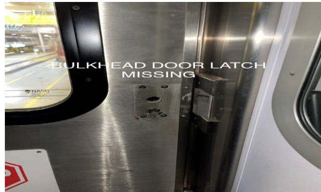
Picture 14: Cannibalized Door Latch
