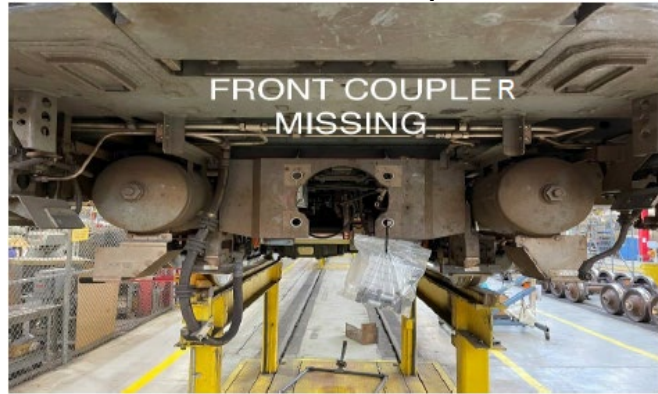
Picture 3: Cannibalized Front Coupler
