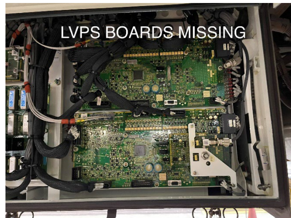
Picture 5: Cannibalized LVPS Boards
